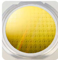
Wafer diced on frame
